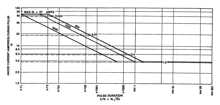
Solid lines represent constant repetition rates. Dashed lines represent constant duties. Do not extrapolate above or to the right of bold lines which set boundaries of maximum anode current and minimum repetition rate, respectively.
