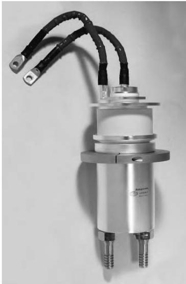
Flying filament leads with coaxial grid ring — integral water jacket
